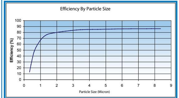
Performance data is based on the ASHRAE 52.2-2007 Test Methods, Test velocity 295 FPM for 24x24x1 and 492 FPM for 24x24x4 nominal size filters.
